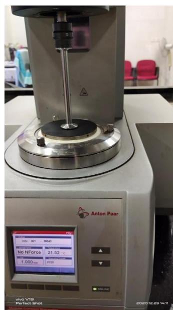
Fig. 1: MCR 52 modular compact rheometer with 25 mm parallel plate type of probe- for analysing viscosity with respect to temperature.
